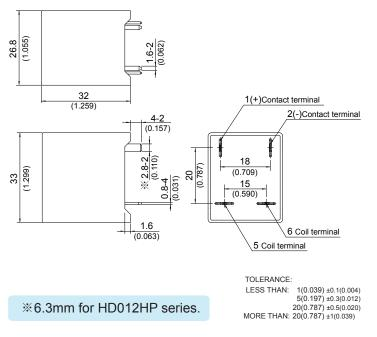
Wiring Diagram (bottom view)
